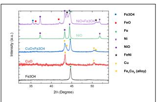
Fig. 1. X-ray diffraction patterns of in-flight reduced  $Fe_3O_4$  particles, CuO particles, CuO- $Fe_3O_4$  mixture, NiO and NiO- $Fe_3O_4$  mixture.
